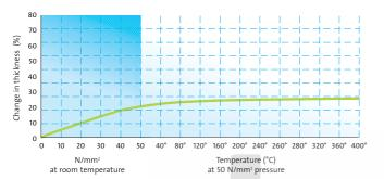
The temperature and pressure recommendations in the graphs apply to gaskets with a thickness of 2.0 mm and smooth flanges. Higher stresses are possible when thinner gaskets are used!
